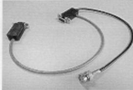
The **TTL cable** (Com 1) is used for connection to both the treadmill/ergometer and Tango.
