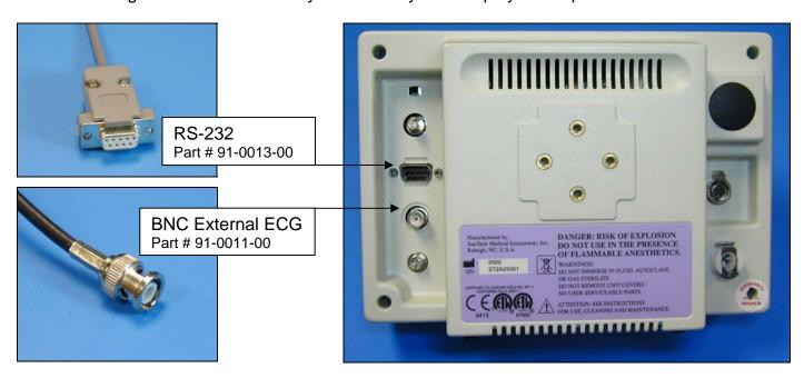
1. Plugging in the ECG trigger cable
