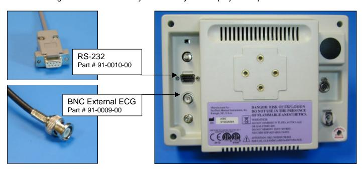
1. Plugging in the ECG trigger cable
