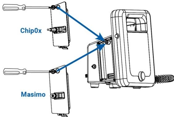
To add an SpO<sub>2</sub> module, attach the module on the left side of the main unit. Fasten with the included Phillips-head screwdriver.
