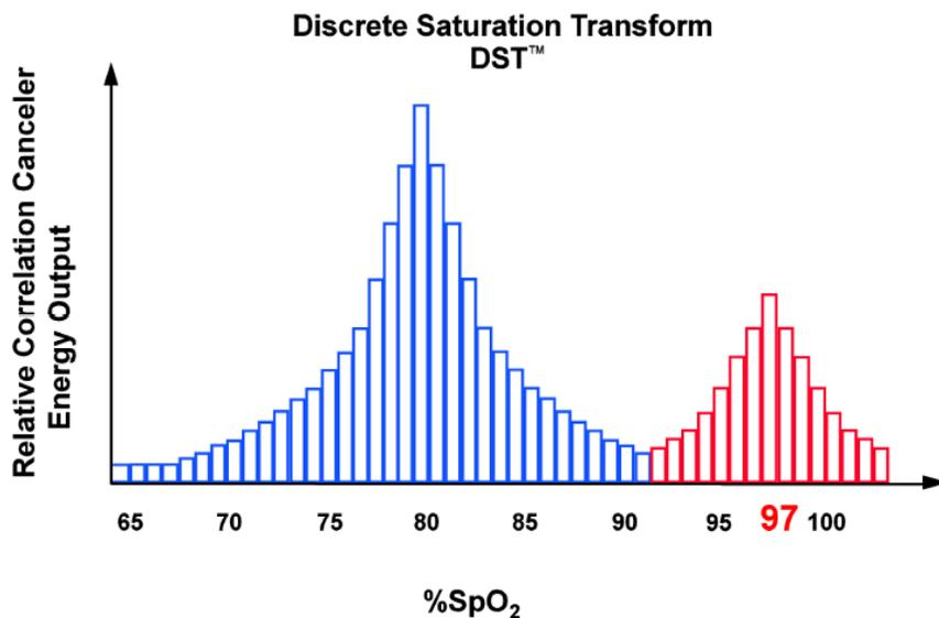
The DST plot has two peaks: the peak corresponding to the higher saturation is selected as the SpO<sub>2</sub> value. This entire sequence is repeated once every two seconds on the most recent four seconds of raw data. The MS board SpO<sub>2</sub> therefore corresponds to a running average of arterial hemoglobin saturation that is updated every two seconds.
