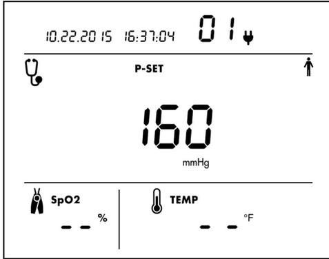
Example shows Auscultatory SphygmMode setup display. Three-digit number is the target cuff inflation pressure setting. The default is 160 mmHg.
