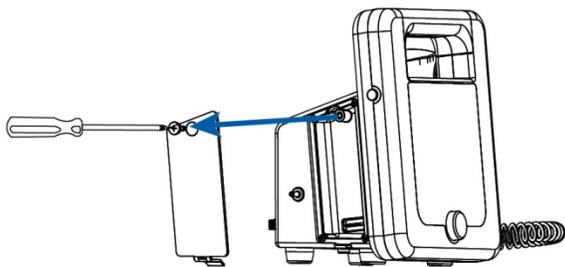
Remove the left panel of the CT40, using a Phillips head screw driver. This panel will be on the left side, when the screen is facing the user.
