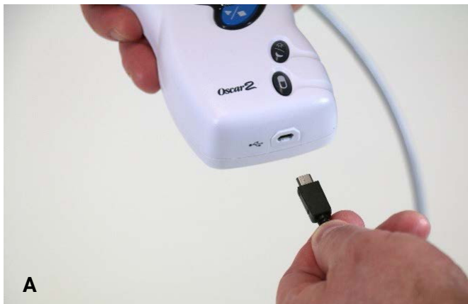
Figure 1: Connecting the Oscar 2 to a PC
