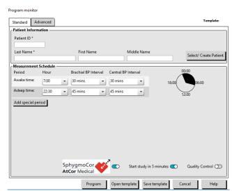
Figure 3: Programming the Oscar 2 (Standard Tab)
