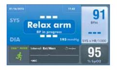
Once the stress test begins, the stress system will prompt the monitor to take blood pressure readings. The cuff will automatically inflate for each measurement. The message "RELAX ARM BP in progress" will be displayed until the measurement is complete, then the reading will be displayed. You can also press the START/STOP button to manually prompt the monitor to take blood pressure readings. This same button can be used to abort a reading if necessary.
