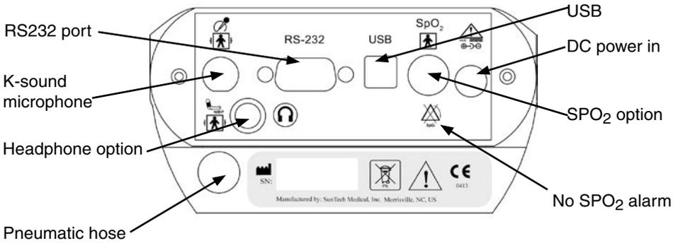
Figure 1: Connector Panel Connections
