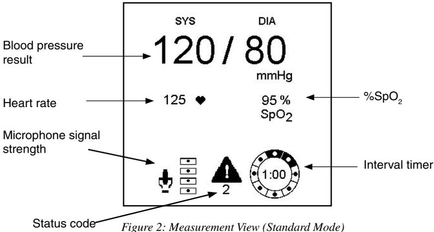
Figure 2: Measurement View (Standard Mode)
