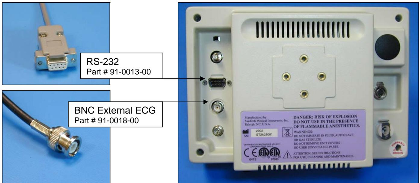
1. Plugging in the ECG trigger cable
