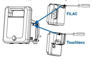
To add a temperature module, attach the module on the right side of the main unit. Fasten with the included Phillipshead screwdriver.
