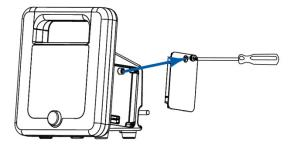
If no temperature module will be added, then attach the right panel of the CT40, using the included Phillips-head screwdriver. This panel will be on the right side, when the screen is facing the user.
