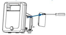
If no temperature module will be added, then attach the right panel of the CT40, using the included Phillips-head screwdriver. This panel will be on the right side, when the screen is facing the user.
