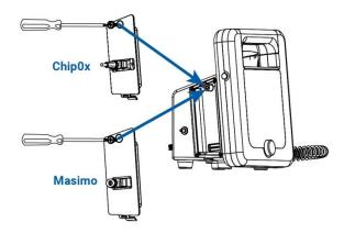
To add an  $SpO_2$  module, attach the module on the left side of the main unit. Fasten with the included Phillips-head screwdriver.
