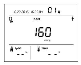
Example shows Auscultatory SphygMode setup display. Three-digit number is the target cuff inflation pressure setting. The default is 160 mmHg.
