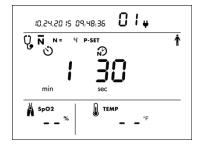
You can select 2 to 5 measurements to average\*. In this example, 4 measurements are set to be averaged.
