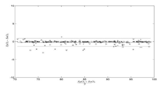
The tested device meets the stated accuracy specification of RMS Error = 2.00% for the range 70% to 100% SaO<sub>2</sub>. The accuracy is not specifed below 70% SaO<sub>2</sub>. In addition, here are detailed measured A<sub>RMS</sub> values over the specified discreet ranges:
