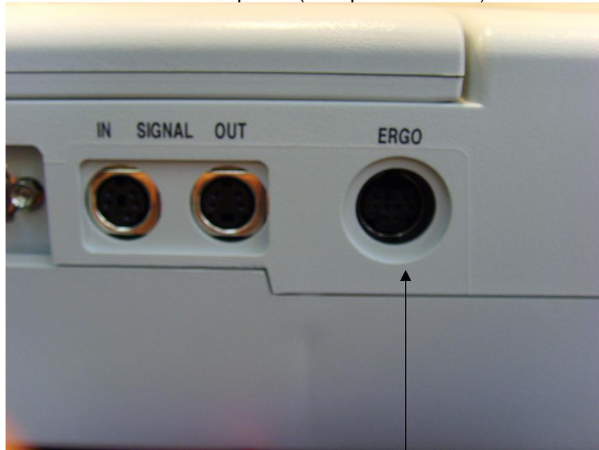
ECG Trigger Connection
