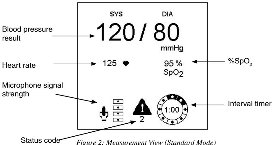
Figure 2: Measurement View (Standard Mode)
