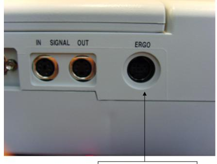
ECG Trigger Connection
