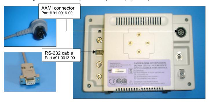
1. Plugging in the ECG trigger cable
