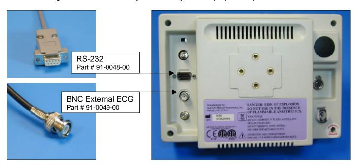
1. Plugging in the ECG trigger cable
